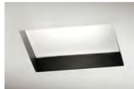
←↓ T382 Filiatrà Recessed plaster spotlight with black painted inner edge and opal glass GX53 – 1x10W w80 x d80 mm lighted hole
