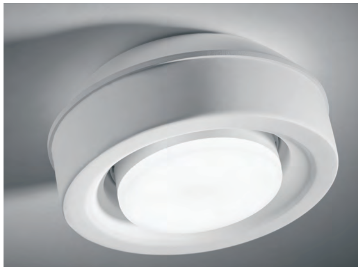
↓ → T571 Ellade Plaster ceiling lamp for indirect lighting with matte white painted element GX53 – 1x10W Ø125 x h54 mm
