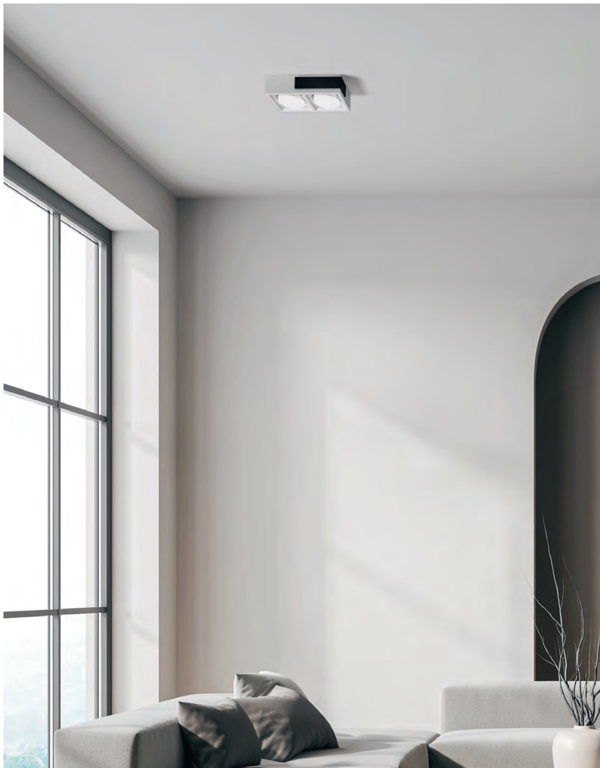
↑ → T546 Velia Plaster ceiling lamp for indirect lighting with matte black painted elements GX53 – 2x10W w218 x d115 x h55 mm
