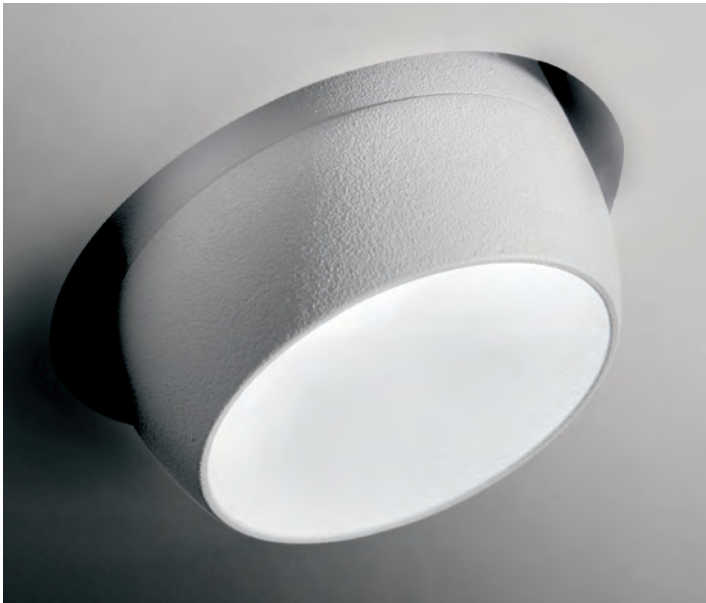
↑ → T412 Lelanto One-light adjustable recessed plasterboard spotlight with matte white painted ring finishing. Adjustable 15° tilt light. GU10 – 1x10W Ø50 mm aluminium ring Technical data 447
