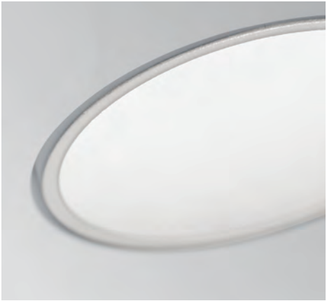
←↑ T391 Thessaly Raso Flush recessed plaster spotlight with matte white painted ring finishing GU10 – 1x10W Ø60 mm aluminium ring Technical data 441
