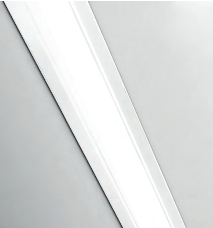
↓ → T221.W Oropus White coated extruded aluminium system with satin cover w25 x h18,5 mm lenght: 500/1000/1500/2000 mm
