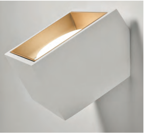
↓ → T436 Nasso quadrata Plaster wall lamp for indirect lighting with satin brass frame finishing GX53 – 1x10W w120 x d120 x h140 mm Technical data 475
