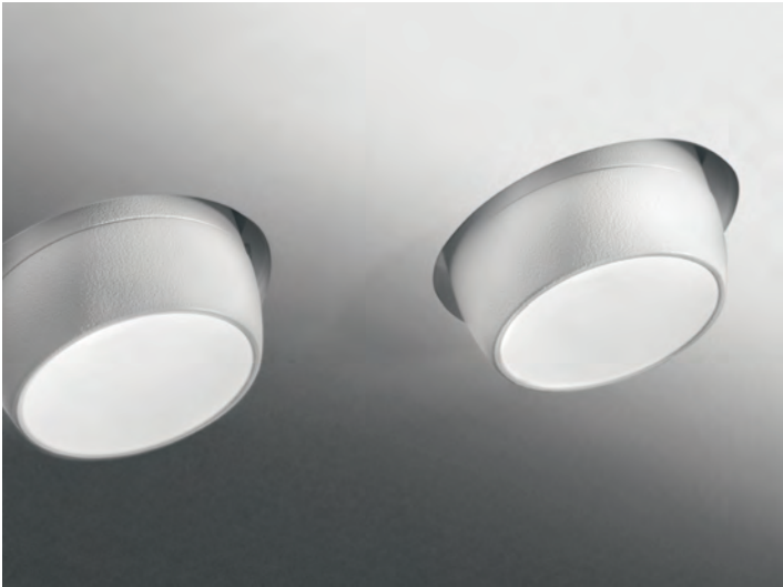
← ↓ T413 Lelanto Two-lights adjustable recessed plasterboard spotlight with matte white painted rings finishing. Adjustable 15° tilt light. GU10 – 2x10W Ø50 mm double aluminium ring Technical data 447
